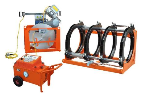
The **DELTA 800 Easy Life** is a hydraulic mirror welding machine, suitable for welding pressure piping systems for water, gas, or other media. The machine has a range of **500 to 800 mm** and is built according to international standards (UNI 10565, ISO 12176-1). Thanks to the special control box, the machine can handle a semi-automatic welding process.
