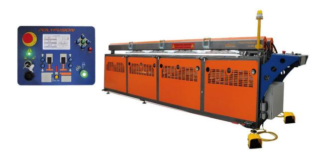
The **POLYFUSION 3-30** is a **3-meter** wide and easy to use hydraulic mirror welding machine, suitable for welding plastic sheets up to **30mm thickness.** The welding process is CNC controlled by a PLC, which works according to DVS 2207. The machine can weld straight sheets together, perform 90°corner classes and weld cylinders from sheets.
