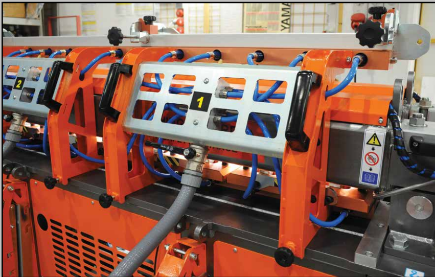
Vacuum holding system sheets supports
