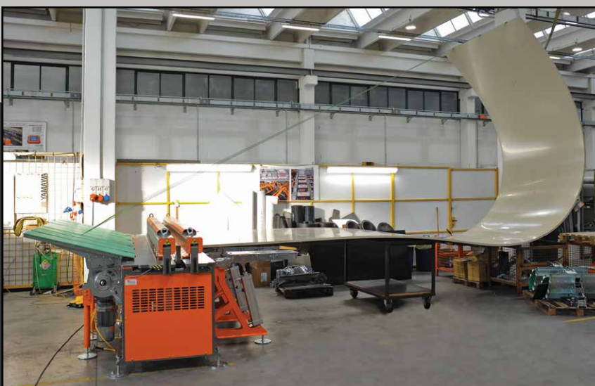
Pulling belts in action
