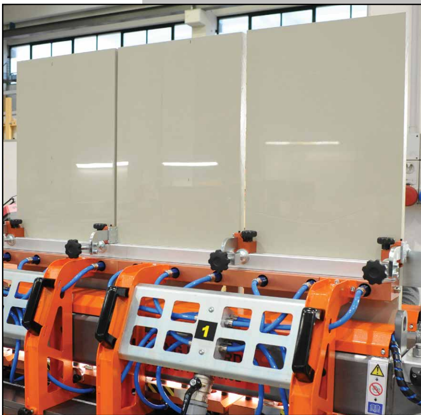
Sheet in place and ready to be welded
