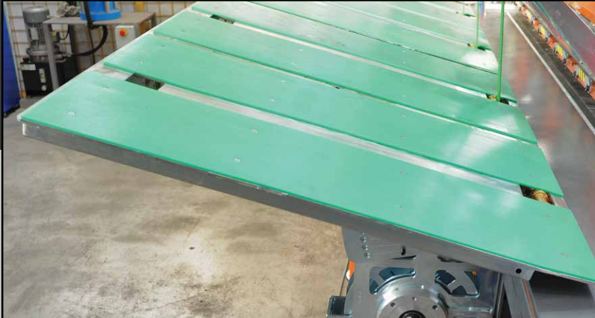
Flat slides for sheets higher 15 mm to roll in place
