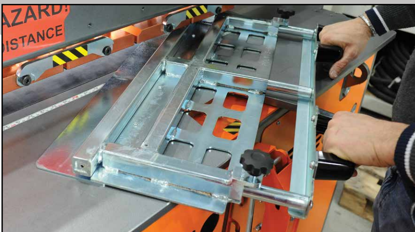
Horizontal positioning frame
