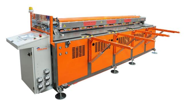
The **POLYFUSION 4** is a **4-meter** wide and easy-to-use pneumatically driven mirror welding machine, suitable for welding plastic **sheets** up **to 50mm thickness (double wall 60mm).** The welding process is CNC controlled by a PLC, which works according to DVS 2207. The machine can weld straight sheets together, perform 90° corner classes and weld cylinders from sheets.
