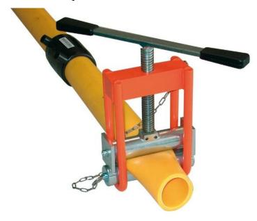
The **SQUEEZER 63** is a manual tool. Easy to use on site, it can stop the gas or water flow in polyethylene pipes from **16 to 63 mm, SDR 11 and SDR 17.**
