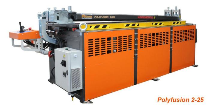
The **POLYFUSION 2-25** is a **2-meter** wide and easy to use manual hydraulic mirror welding machine, suitable for welding PE and PP **sheets** up **to 25mm thickness.** The welding process is handled by a control panel that operates a hydraulic control box. This control panel can be moved horizontally.
