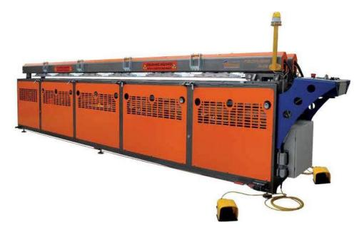
The **POLYFUSION 4-30** is a **4-meter** wide and easy to use hydraulic mirror welding machine, suitable for welding plastic sheets up to **30mm thickness.** The welding process is CNC controlled by a PLC, which works according to DVS 2207. The machine can weld straight sheets together, perform 90°corner classes and weld cylinders from sheets.
