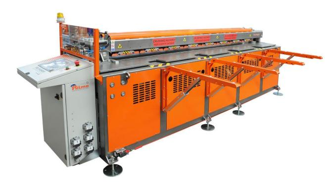
The **POLYFUSION 3** is a **3-meter** wide and easy-to-use pneumatically driven mirror welding machine, suitable for welding plastic **sheets** up **to 50mm thickness (double wall 60mm).** The welding process is CNC controlled by a PLC, which works according to DVS 2207. The machine can weld straight sheets together, perform 90° corner classes and weld cylinders from sheets.
