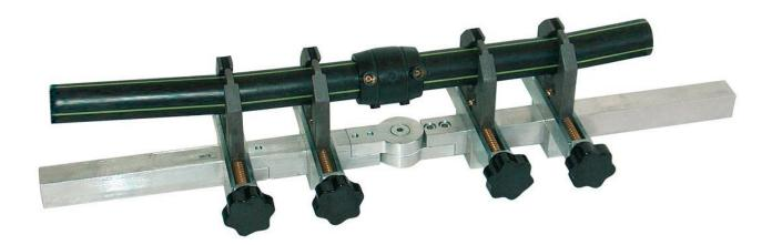
This professional tool is essential to keep pipes aligned during electro welding. The "UNIVERSAL ALIGNER 63" is almost entirely made of a special alloy and has a centrally adjustable connection to form 45° and 90° angles. It has 4 self-centering clamps that do not require adapters. It is possible to remove 1 part of the shaft, and 1 clamp, to be able to weld tees.
