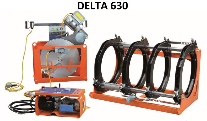
The **DELTA 630** is a manual hydraulic mirror welding machine, suitable for welding pressure pipe systems for water, gas, or other media. The machine has a range of **280 to 630 mm** and is built according to international standards (UNI 10565, ISO 12176-1).
