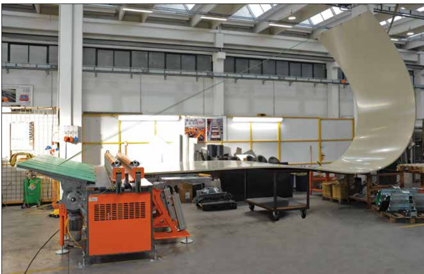
Pulling belts in action
