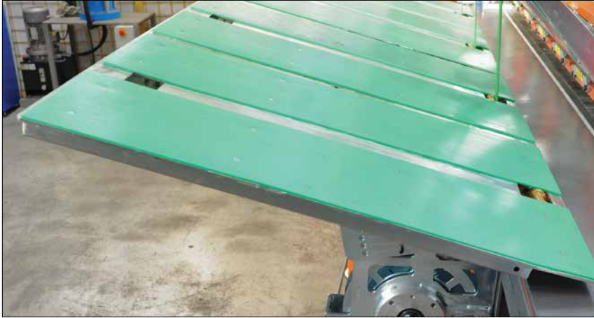
Flat slides for sheets higher 15 mm to roll in place
