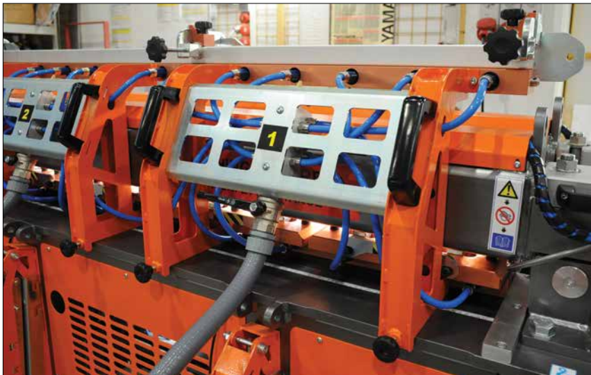
Vacuum holding system sheets supports
