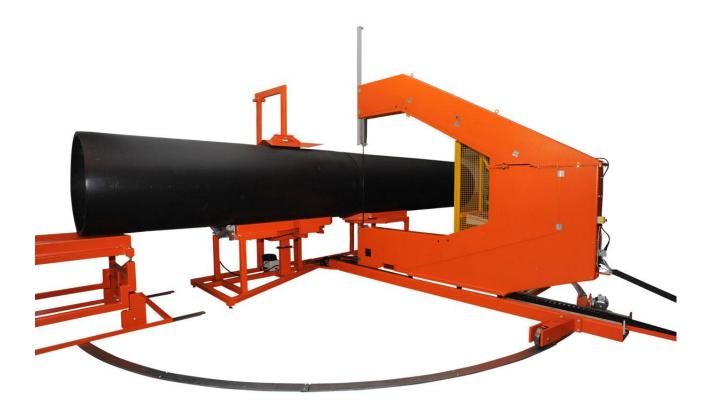
The **SIGMA 1200 PRO** is an electric band saw machine for the workshop. This machine can saw HDPE, PP, PVDF and PVC. The **SIGMA 1200 PRO** was developed to create angular saws with a wide range (-45° to 67.5°). Both the preparation and the sawing phase itself are extremely simple and safe to carry out.
