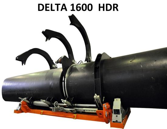
The **DELTA 1600 HDR** is a manual hydraulic mirror welding machine, suitable for welding pressure piping systems for water, gas, or other media. The machine has a range of **800 to 1600 mm** and is built according to international standards (UNI 10565, ISO 12176-1).
