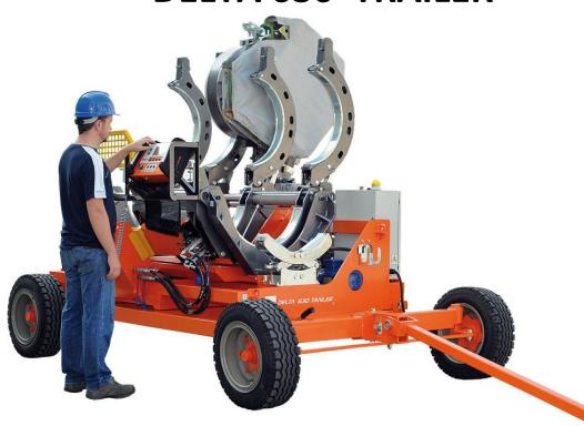
The **DELTA 630 TRAILER** is a self-aligning hydraulic mirror welding machine, suitable for welding pressure pipes for water, gas and other liquids, for diameters **225\*** up **to 630 mm.** This aircraft operates according to the international standards ISO 21307 HIGH PRESSURE and ASTM F2620. The **DELTA 630 TRAILER** has no generator on board and needs external power.
