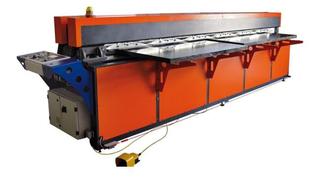
The **POLYFUSION 4-50** is a **4-meter** wide and easy-to-use hydraulic mirror welding machine, suitable for welding plastic **sheets up to 5 0mm thickness.** The welding process is CNC controlled by a PLC, which works according to DVS 2207. The machine can weld straight sheets together, perform 90° corner classes and weld cylinders from sheets.
