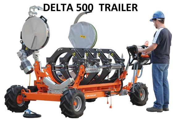
The **DELTA 500 TRAILER** is a self-aligning hydraulic mirror welding machine, suitable for welding pressure pipes for water, gas and other liquids, for diameters **200 to 500 mm.** This aircraft operates according to the international standards ISO 21307 HIGH PRESSURE and ASTM F2620. The **DELTA 500 TRAILER** does not have a generator on board and needs external power.
