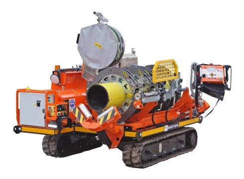
This welding machine is used on location, it has a low-vibration diesel engine and has tracks. The machine is suitable for welding plastic pressure pipes for transport of water, gas and other liquids. It can handle pipes with a diameter of **250 to 500 mm** and was built according to international standards.
